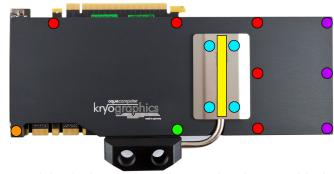
Attach back plate and graphics card to the water block. To do so, use the following mounting material depending on the colored markings in the figure:
