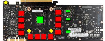
Clean the surfaces of all RAM modules on the back side of the graphics card using benzine if necessary. Apply a thin layer of thermal compound to the RAM modules on the back side, marked red in the figure. The thermal compound must not be electrically conductive!
