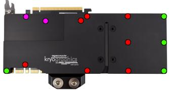
Red marking: seven screws M3 x 10 mm. Violet marking: two screws M3 x 8 mm. Green marking: four screw M3 x 6 mm.
