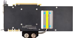
pipe and fasten the plate using four screws M3 x 5 mm (marked blue in the figure). Step 9:
