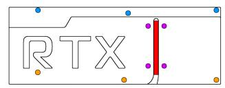
Blue marking: Three screws M2,5 x 8 mm, countersunk head.
