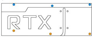
Blue marking: Three screws M2,5 x 8 mm, countersunk head.
