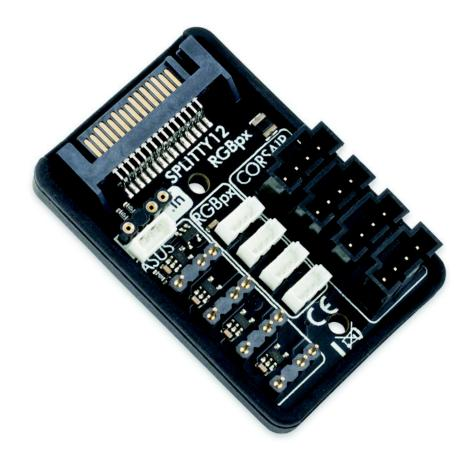
This splitter can be used to connect up to 12 RGBpx/ARGB components to a single RGBpx or ARGB output. All twelve outputs are connected in parallel, all connected components are controlled identically. Power for all outputs is supplied through a SATA power connector.
