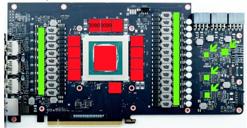
Apply a thin layer of thermal compound to the GPU and the RAM modules (ten RAM modules for 3080, twelve for 3090). These components are marked red in the figure. Place the pre-cut thermally conductive pads supplied with the kryographics on top of the components as indicated by green rectangles.
