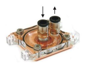
Unlike channel coolers, the nozzle- and microstructure coolers cuplex XT, cuplex hd and cuplex PRO have a predefined flow direction. For the cuplex PRO, the water must be led in through the centrical connection directly onto the microstructure, in the case of cuplex XT and cuplex hd, the water is to be led in through the fitting connected to the
