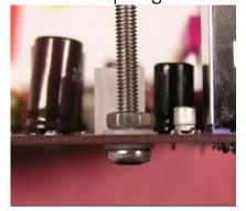
that purpose detach your motherboard from the computer case. In P4- and Xeon-systems the mostly black plastic mounting for air-coolers has to be removed from the motherboard to reveal the necessary drill holes on it. Next slide a plastic washer over one of the supplied stainless steel M4 screws which you then put through the holes adjacent to the socket from
