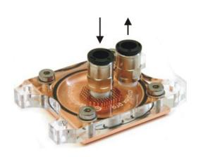
Unlike channel coolers, the microstructure coolers cuplex kryos and cuplex PRO have a predefined flow direction. The coolant must be led in through the central connection directly onto the microstructure, the coolant is then led out through the lateral connection. In order to attain the full performance of the waterblock, correct connection of inlet and
