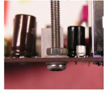
that purpose detach your motherboard from the computer case. In P4- and Xeon-systems the mostly black plastic mounting for air-coolers has to be removed from the motherboard to reveal the necessary drill holes on it. Next slide a plastic washer over one of the supplied stainless steel M4 screws which you then put through the holes adjacent to the socket from below. Slide
