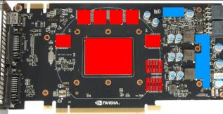
Apply a thin layer of thermal compound to the GPU and the RAM modules. These components are marked red in the figure. The RAM modules markes with red stripes are not present on every card, thermal compound should only be applied if RAM modules are present. The thermal compound must not be electrically conductive! Cut fitting pieces from the thermally conductive pad supplied with the aquagraFX and place them on top of the voltage regulators as indicated by blue rectangles.
