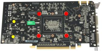
the figure. Use extreme caution not to damage any of the highly sensitive components of the graphics card! Disconnect the fan connector while lifting the air cooling unit off the graphics card.
