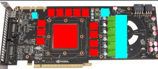
the voltage regulators as indicated by blue rectangles. Take care not to miss the component on the left side of the figure! An additional thermally conductive pad (thickness 1 mm, not included in delivery) can be placed in the green marked area.
