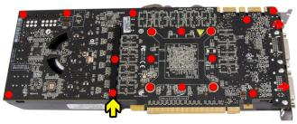
caution not to damage any of the highly sensitive components of the graphics card! Disconnect the fan connector while lifting the air cooling unit off the graphics card. The foam strip indicated by a yellow arrow should be removed.
