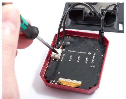
Insert one stripped motor power lead into each of the two cable clamps on the controller board while pressing down the corresponding release tab using a small screwdriver or a ball point pen (see figure). There is no polarity to respect.
