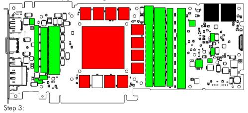
Attach the kryographics Pascal for RTX 2080 Ti to the graphics card. To do so, at first carefully and evenly screw in the four screws adjacent to the GPU, afterwards the remaining screws (sixteen screws M2,5x4 mm).
