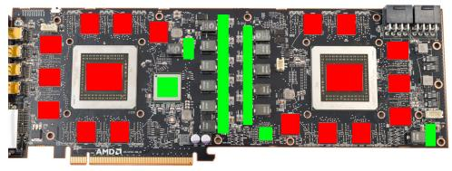
Apply a thin layer of thermal compound to the GPUs and the RAM modules. These components are marked red in the figure. The thermal compound must not be electrically conductive! Cut fitting pieces from the thermally conductive pad supplied with the kryographics and place them on top of the voltage regulators and PCle switch as indicated by green rectangles.
